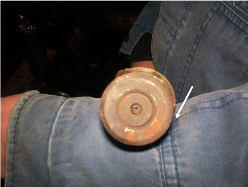
Clean cut surface of the boiler nozzle when operating on fuel treated with **PowerFuel®** technology.
